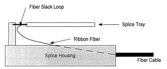
Improper Fiber Slack Storage Diagram
