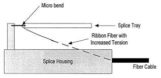
Improper Fiber Slack Storage Diagram
